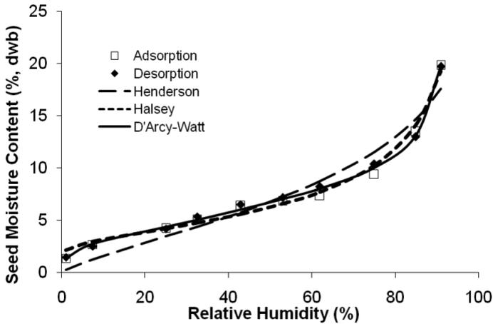
Figure 4. Equilibrium moisture content of drumstick tree seeds predicted by modified Henderson, modified Halsey, and D'Arcy-Watt equations compared to the actual data.
